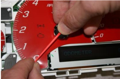
16. Press down with your thumb on the center of the hub. ONLY 1/2 down for now.
