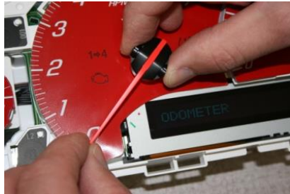
21. If a needle is set wrong, remove it. Unplug the cluster and start over.
