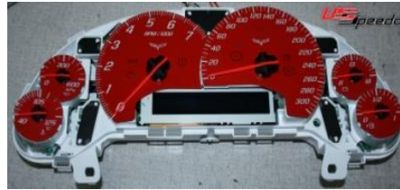
18. Now you should have all the needles in place. Unplug and put the cluster in your lap.
