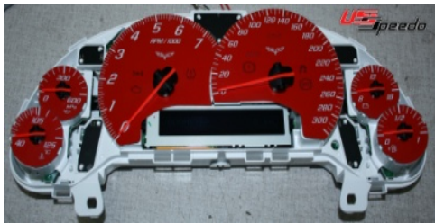
20. Plug the cluster back in, each needle should go back to the low or 0.
