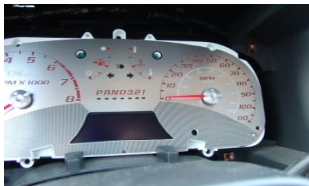
13. Place the needles in place. Set each needle at 0 or low.
