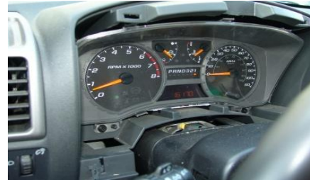
2. The trim is only held in with clips, just pull out.
