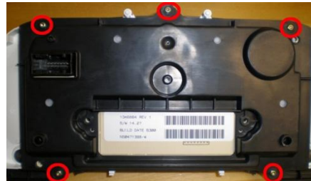
6. Remove the screws on the back of the cluster.
