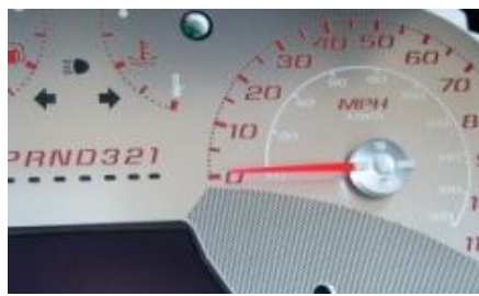
14. Do not push the needles all the way down yet.
