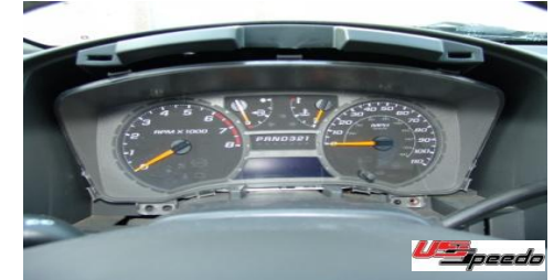
3. Remove the 4 7mm screws. Mark the needle locations on the diagram below. Leave key off.
