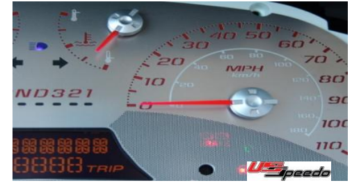
19. Make sure the needles go back to 0 or low and install.
