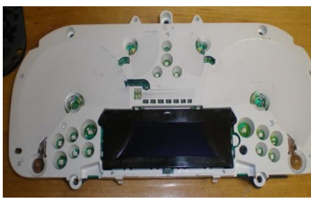
5. Take the cluster inside to remove the gauge face.
