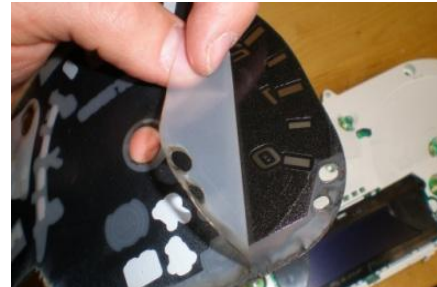
10. On the back of the US Speedo gauge face is plastic liner, remove.
