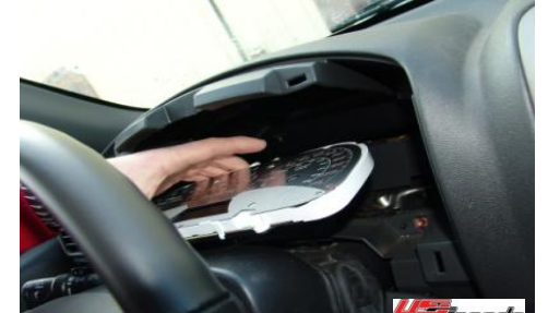
11. Place the gauge face in place and take back to the truck and plug in.
