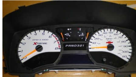
5. Take the cluster inside to remove the gauge face.
