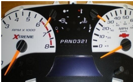
8. Twist each needle down past the low marks. And remove.
