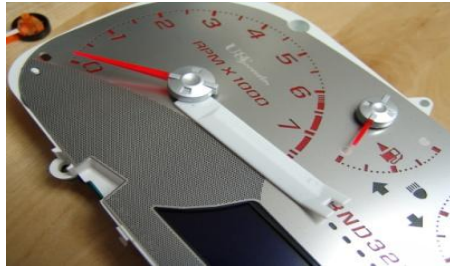
17. Take the cluster out and place on flat surface. Slide the handle of the needle tool under the hub of the needle and push down.
