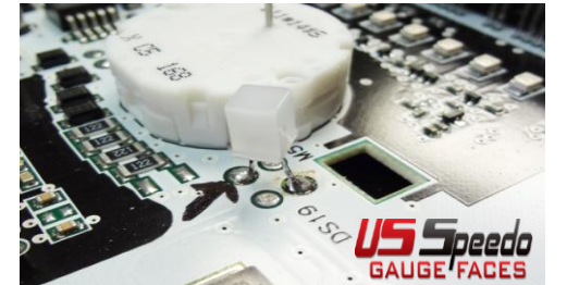
7. Heat up one pad and mount one side of the CUBE Bent leg goes towards the black mark.
