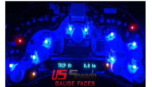
11. Make sure each LED is lighting correctly.
