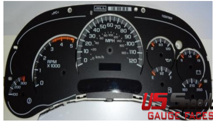
1. Remove the needles and take cluster apart. Refer to US Speedo Gauge Install.
