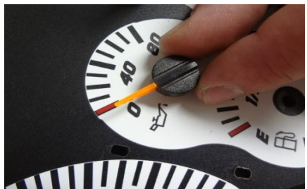
14. Set each needle exactly as before you removed them.
