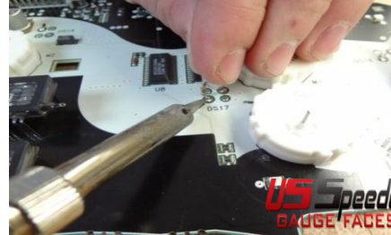
6. Put a bit more solder on the 2 pads to be used.
