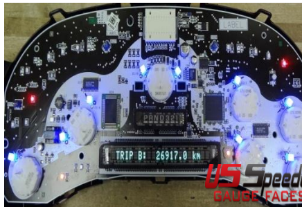
10. Plug the cluster in, and make sure each LED is working correctly.
