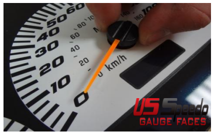
13. Follow the US Speedo gauge install to reset the needles.
