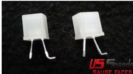
4. The new Cube LEDs has 2 legs, one straight, one is bent
