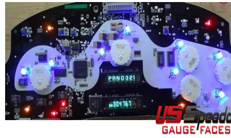
10. Plug the cluster in, and make sure each LED is working correctly.
