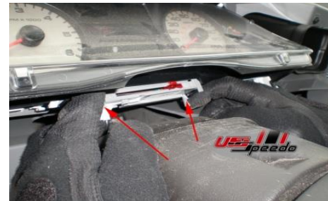
8. Remove the shift indicator. Push in on the tabs and slide down.
