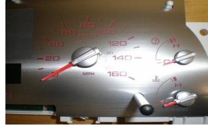
27. Take the cluster back to the truck and plug in. Make sure each each is correct and install.
