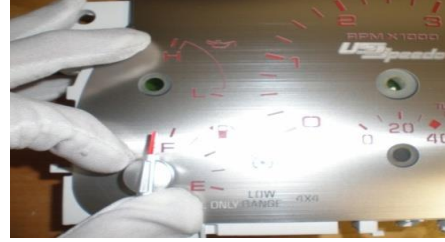
22. Unplug the cluster. Twist each needle 1/2 way up. Plug in.
