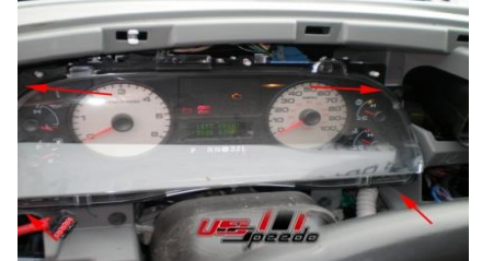
7. Remove the 4 -7mm screws hold the cluster in place.
