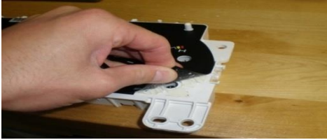
16. Remove the factory gauge face. It has glue on the back side.
