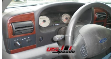
1. Pull on the dash to remove. It is held in place with clips.
