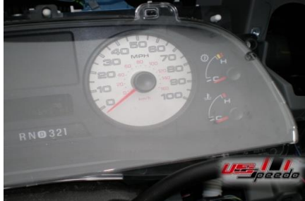
9. Turn the key on then off. Mark each of the needle positions on a piece of paper.
