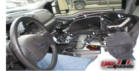
6. Pull the dash over the steering wheel and toward you. You don't need to remove all the switches.
