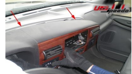
3. Reach behind the dash and unplug the switches.
