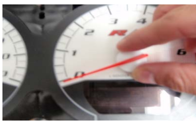
Take the cluster back to the car, plug it in, and with the key off, place the needles where they are marked on diagram.
