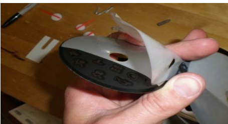
Remove the plastic backing on the new face and place the face onto the cluster.
