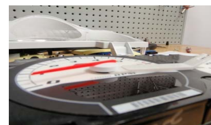
Unplug the cluster and check needle height with tool provided as shown.
