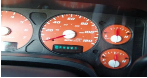
16. Unplug the cluster and plug back in. If the needles are set wrong, remove and start over.
