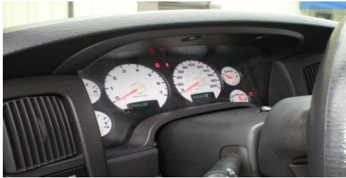
Mark the position of each needle with the key off.
