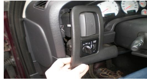
2. Pull on the left side vent. It is held in by clips.
