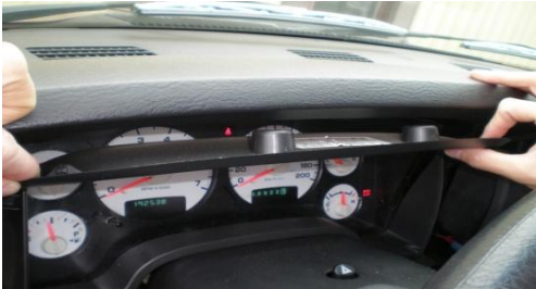
4. Pull the trim around the speed off. Some may have a screw on each side.
