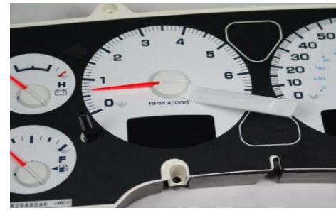
10. Use the needle tool to remove the needles.
