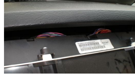
14. Take the cluster back to the truck and plug in. Leave key OFF
