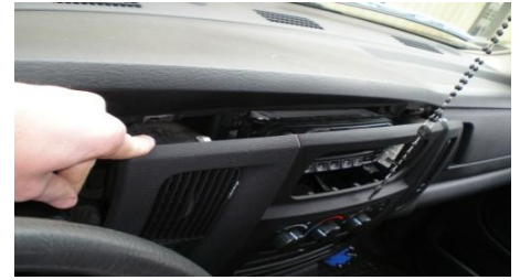
3. Pull on the right side vent and trim. It is held in by clips.
