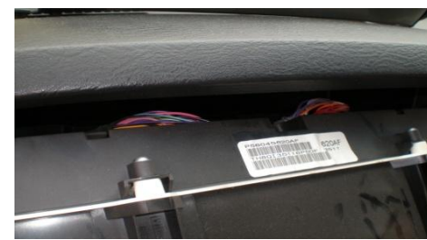
6. There are 2 plug in the back of the cluster.
