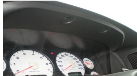
1. Remove the two screws above the cluster.
