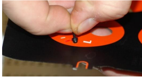
17. Remove the cluster and go back in side to place the needles stop and lens on.
