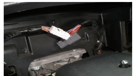
7. You may need to use a screw driver to release the plugs.
