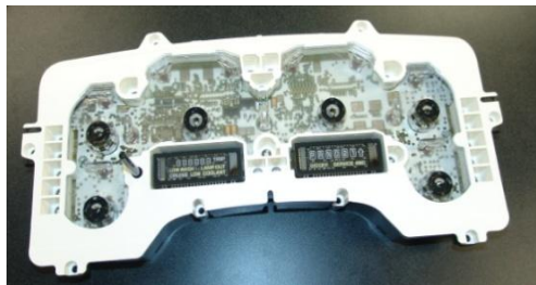
12. It will leave small dimples around the needle hubs, use a knife to remove.
