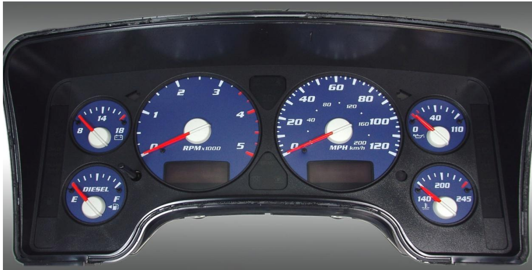
Correct Needle position with the key off.
