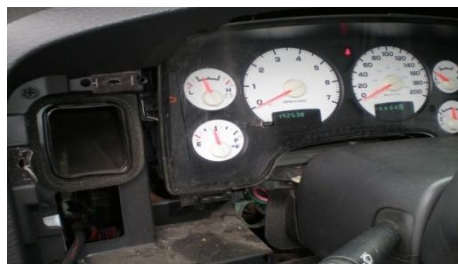
5. The cluster is held in by 4 screws. Remove
