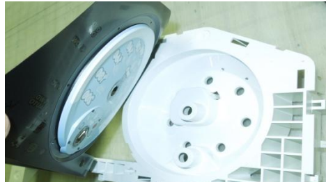
21. Remove the Gauge face and replace with the new US Speedo Gauge Face.
