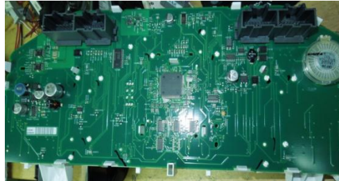
17. Press on the tabs around the outside to remove the board from the plastic.
