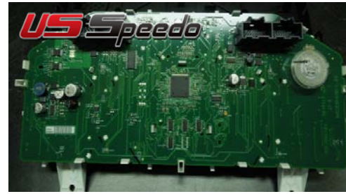
3. Snap the circuit board back into place. Ensure each snap is in.
