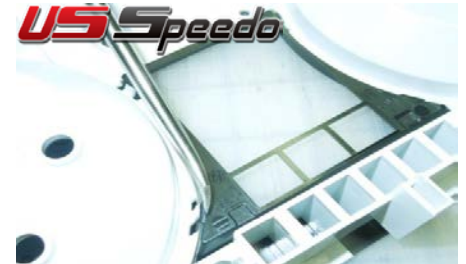
19. Back side center trim. It is held in with clips. Press in to release the clips.
