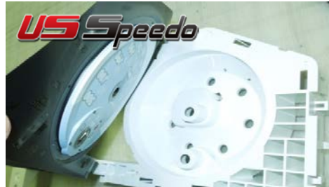
21. Remove the Gauge face and replace with the new US Speedo Gauge Face.
