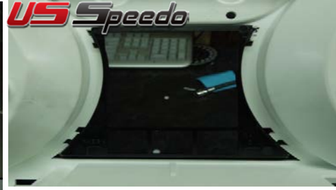
2. Snap the center trim piece into place. Very Snug fit!
