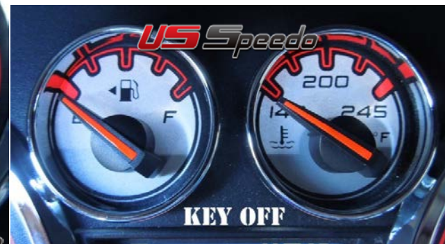
10. When you have all the needles on. Unplug the cluster and plug back in. Check to ensure each needle is EXACTLY as shown here.
