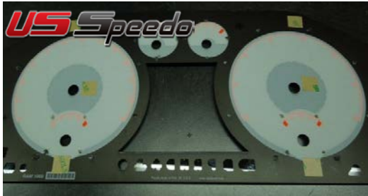
1. Depending on the style of gauge face, remove the back of the top squares.
