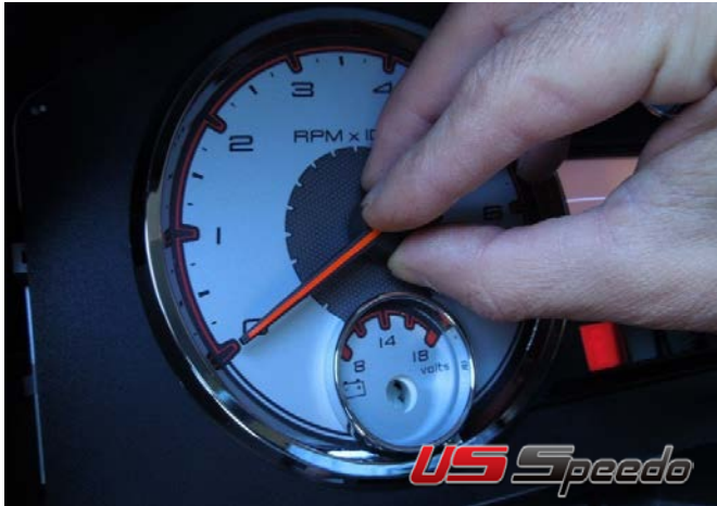
5. With the key ON. Set the Tach Needle as shown. DO NOT twist the needle after it starts to stick on the shaft.
