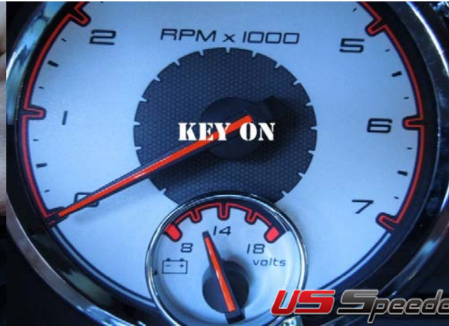
6. Set the Volt gauge if your cluster has one as shown.
