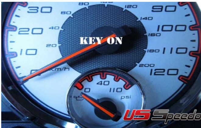
8. Set the Speed and Oil needle as shown with the key ON.
