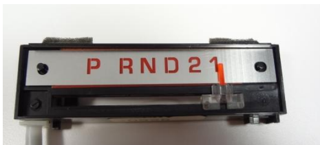
24. On the back side of the new part, remove the liner and put into position
