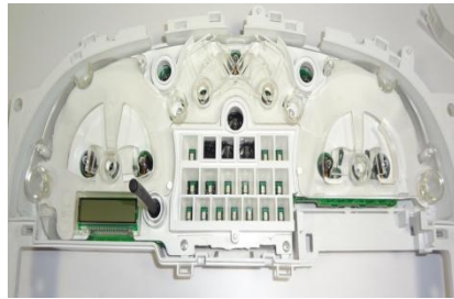
17. Remove each oem gauge face. And put on the cotton gloves
