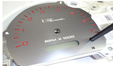
18. Place the new US Speedo Gauge face into position.
