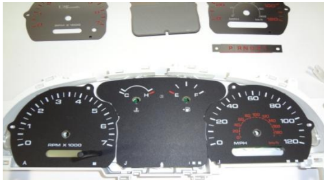
16. Remove each needle. Remove the gauge faces. Notice the little tabs that hold each piece into position.
