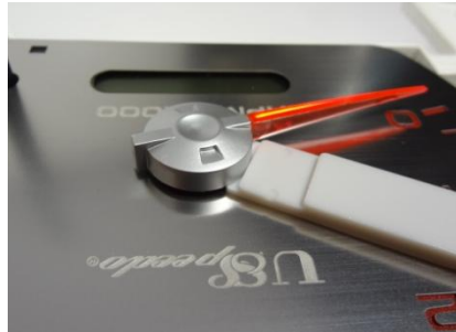
21. Remove the cluster and use the handle of the tool as a height gauge tool. Lowest setting on the handle.
