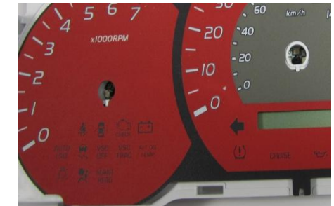
7. Use the needle tool to remove the needles.
