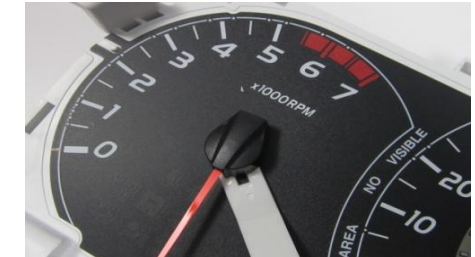
7. Use the needle tool to remove the needles.
