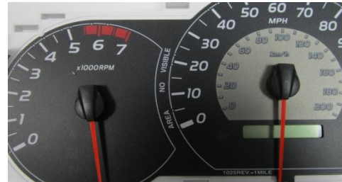
6. Twisting the needles down will help with the removal.
