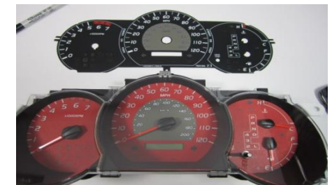
15. Test the cluster before putting the lens back on.
