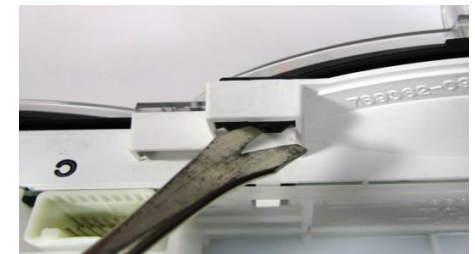
3. Press the tabs from the back side to release the clear top lens.
