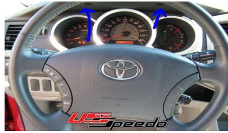
1. Take a picture or mark on the diagram each needle location. KEY OFF
