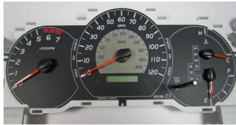
5. With the lens off, twist each needle past the low marks.
