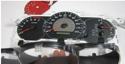
4. Remove the lens and clean if required.
