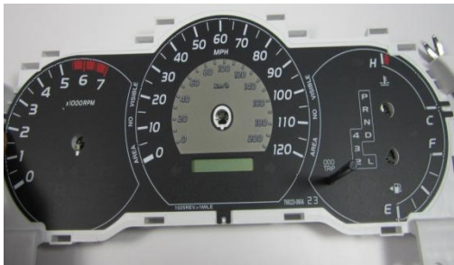
8. Remove each needle. Remove the gauge face CAREFULLY. There are small tabs holding the gauge face
