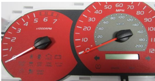
12. Take the cluster back to truck and plug in. Leave the key off and set each needle
