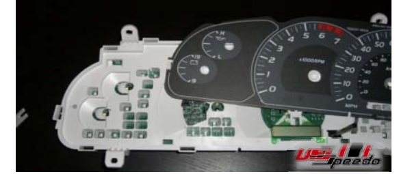
8. Take the cluster inside to a clean place to install the gauge face.
