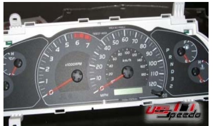
6. Remove the 4 screws holding the cluster in place.
