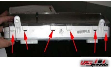
9. Push on the tabs to release the clear lens and black trim.
