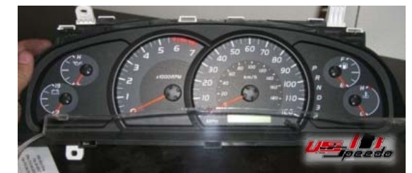
8. Take the cluster inside to a clean place to install the gauge face.
