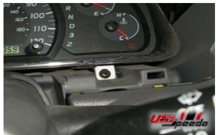
6. Remove the 4 screws holding the cluster in place.
