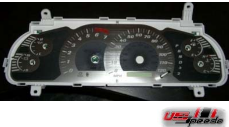
13. Put on the cotton gloves and place the US Speedo gauge face in place.
