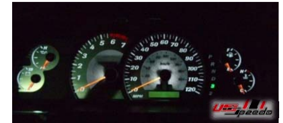
16. Unplug the cluster and plug back in to check each needle position.
