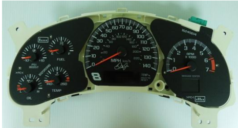
Remove the lense and turn the pointers down past their low point.
