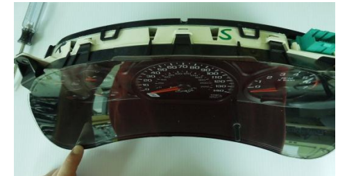
using the screwdriver or clip tool release the clips holding the lens cover on.
