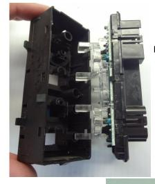
Remove the back of the switch from the front.
