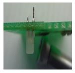
After the holes are clear you can insert the legs of the led though the holes. With the short leg on the side you marked earler.
