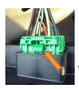
Remove the headlight switch next by releasing the single clip on the top and the two clips on the bottom of the switch. slide the switch out and depress the tab pointed out in the picture to the left to unplug it.
