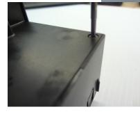
replace the back cover and the four screws. Take the switch back to the vehicle and test its operation.
