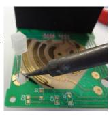
Solder the long leg to its pad. Be sure that the two legs are not touching and that the led is straight up and down and side to side. Bend the legs if necessary.
