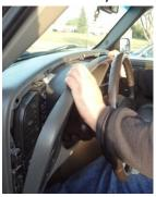
Sharply pull on the front panel of the dash, work your way around until you can lift it up and out, it is only held on by clips and will pop free. place it on top of the dashboard.
