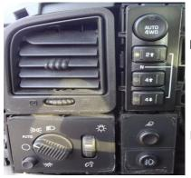
Return the parts back to the vehicle. Plug the headlight switch in first, then slide it into its place. Plug the cargo lamp in and slide it into its place. Plug in both plugs for the 4x4 switch and slide it into its place.
