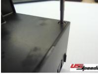
replace the back cover and the four screws. Take the switch back to the vehicle and test its operation.
