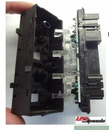
Remove the back of the switch from the front. The circuitboard is permantly attached to the back plastic cover. Remove the clear light pipe.
