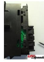
remove the back cover of the switch from the case. The circuit board is not attached to the back. Lift jus the board out of the case leaving the internals inside the case. Be sure to leave the switch face down to prevent pieces from faling out.
