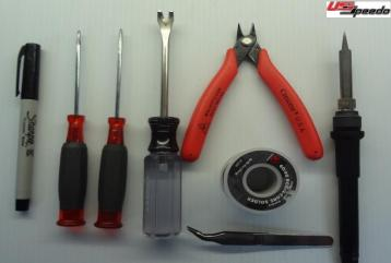
Tools Required Black marker small philips screwdriver small flat screwdriver upolstery clip tool or flat screwdriver small side cutters tweezers solder pencil tip soldering iron
