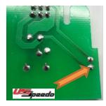
Turn the board over and find the location of the bulb you just cut off. Mark the location shown in the picture to the left.
