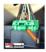
Remove the headlight switch next by releasing the single clip on the top and the two clips on the bottom of the switch. slide the switch out and depress the tab pointed out in the picture to the left to unplug it.
