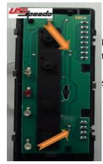
Mark the two pads shown in the picture to the right (very top and bottom). Melt a puddle of solder on the two marked locations. Place the short bent leg into the puddle of solder and align the long leg with its pad before letting the solder cool.
