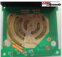
Mark the copper pad that the arrow is pointing to in the picture to the right. This is the pad that the short bent leg will be soldered to.
